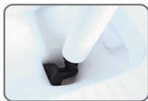
After dipping into the toilet, keep the toilet head vertically to avoid air leakage for better dredging effect.
