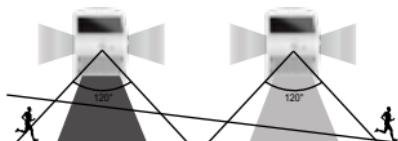
**Mode A:** When battery capacity >30%, lamp automatically turns on to full brightness when motion is detected within the range of ≤6mtrs and then dims to weak brightness(front light ON & back light ON) in 20 seconds of no motion.
