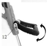
Loosen the adjustment lock knob for the assist handle until it can be moved forwards or backwards without much resistance. Adjust to the desired position and retighten the locking knob.
