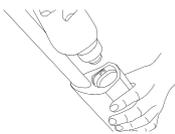
Turn the bottle upside down and press down firmly to snap into place.
