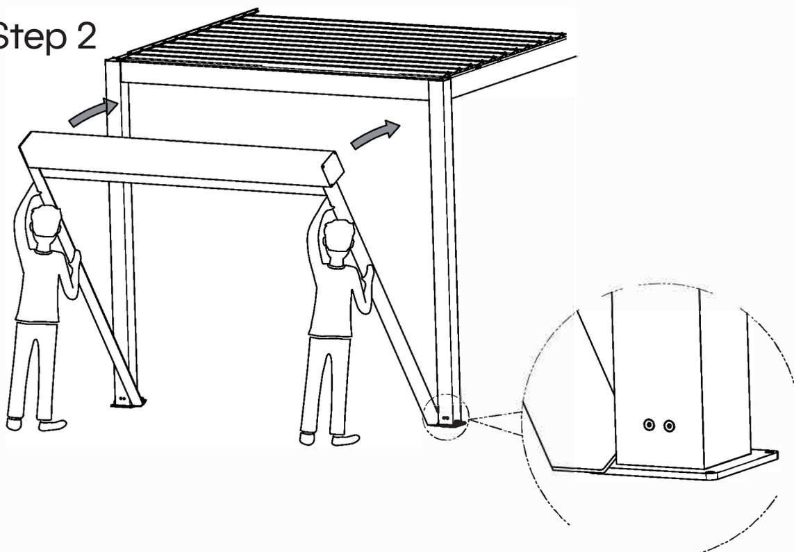
Put the principal module into two columns of pergola for installation, and adjust the position appropriately.
