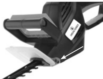
Push the Handle Guard (2) over the blades and fix in place securely with screws on both sides of the housing.
